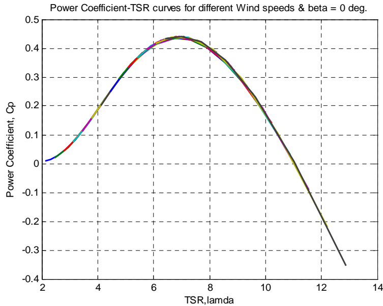
Figure 3.2 Power coefficient vs. tip speed ratio for different wind speeds
