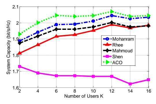
Figure 4.25: Comparison of total system capacity versus number of users for ACO-based algorithm version 3 and other algorithms for  $\gamma_i = 1, \forall i = 1, 2, ..., K$  and 10 ants
