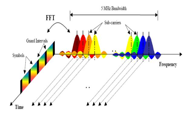
Figure 1.1: OFDM Signal [4]
