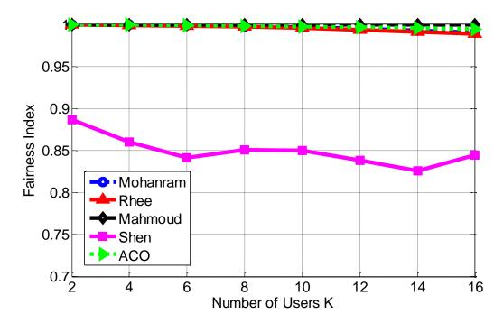
Figure 4.26: Comparison of fairness index versus number of users for ACO-based algorithm version 3 and other algorithms for  $\gamma_i = 1, \forall i = 1, 2, ..., K$  and 10 ants
