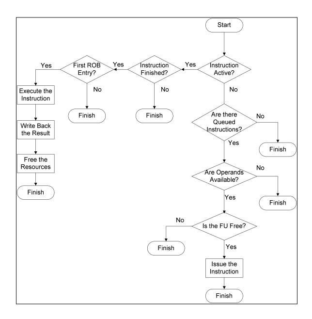
Figure 12: Functional Unit Monitoring Flowchart
