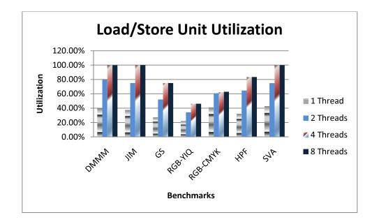
Figure 21: Load/Store Unit Utilization
