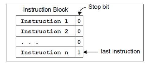
Figure 1: An Instruction Block is Terminating with a Stop Bit
