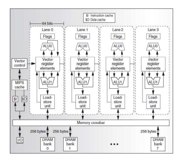
Figure 2: VIRAM Prototype Processor [17]
