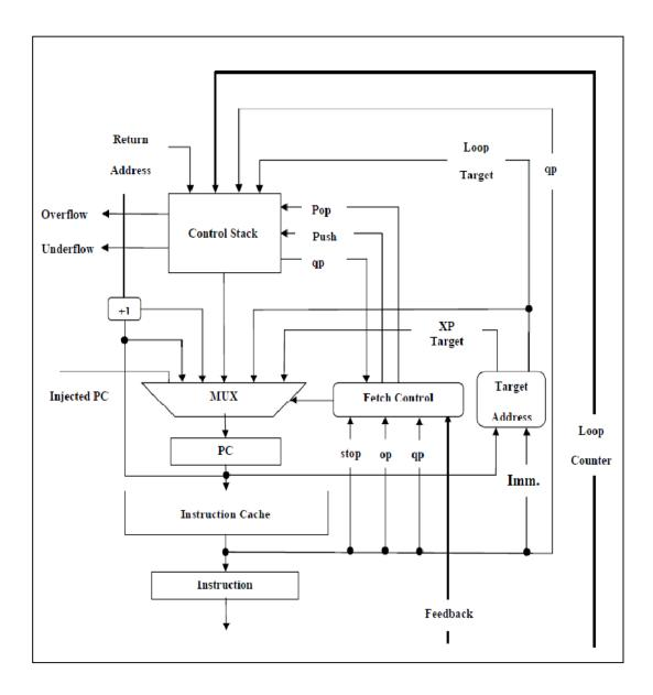
Figure 6: Block Diagram of PAR Core's Frontend
