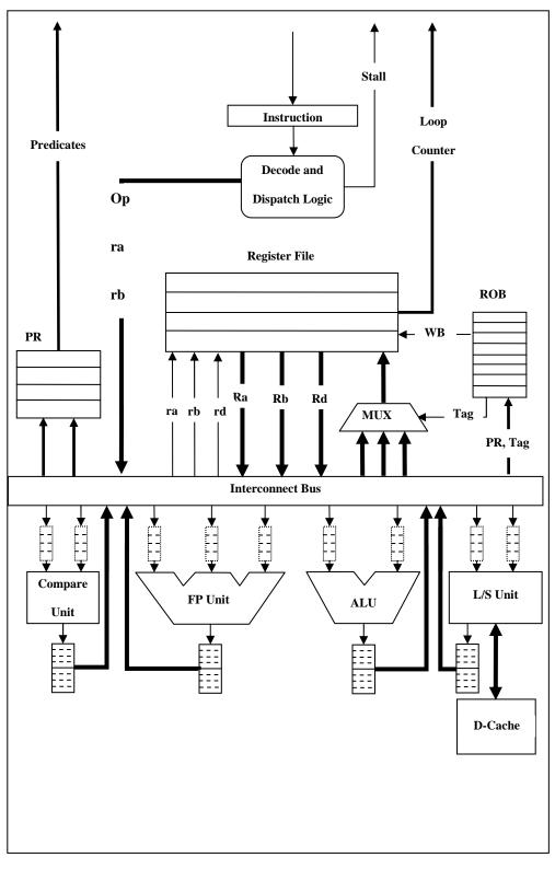
Figure 7: Block Diagram of PAR Core's Backend
