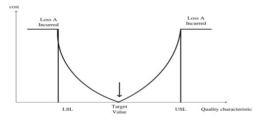
Figure1-2 Taguchi symmetric quadratic loss function
