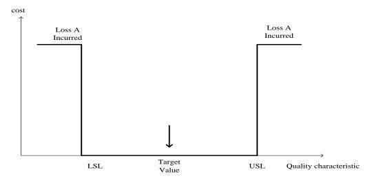
**Figure1-1 Step loss function**
