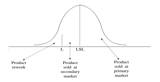
**Figure 2-1 the classifications of the production process**
