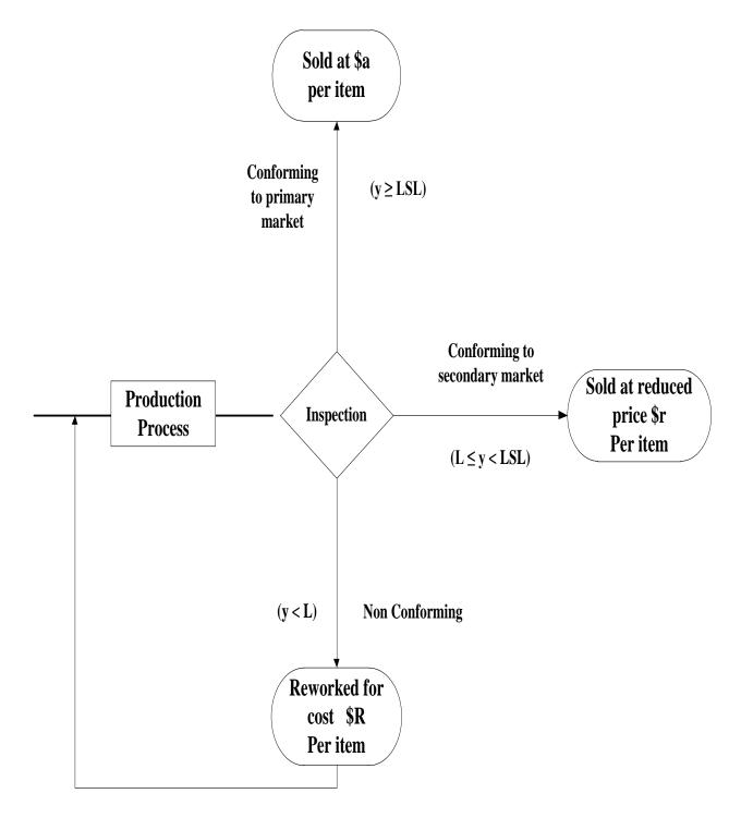
Figure 2-2 The basic production process
