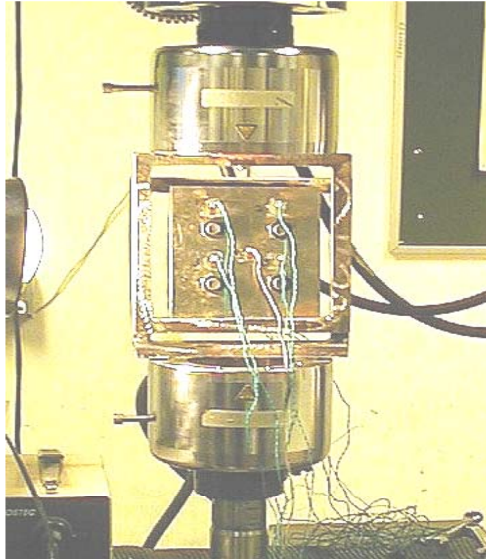
Figure 3.9: Four bolt joint experimental set up
