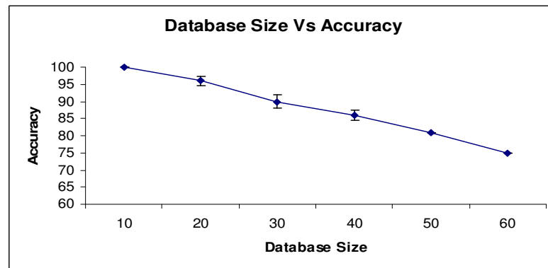
Figure 33: Effect of database size on accuracy in case of similarity transformations and occlusion
