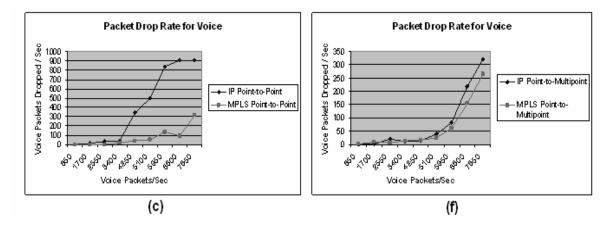
Figure 5.4 Average End-to-End Delay, Inter Arrival Jitter and Drop Rate for only voice traffic.
