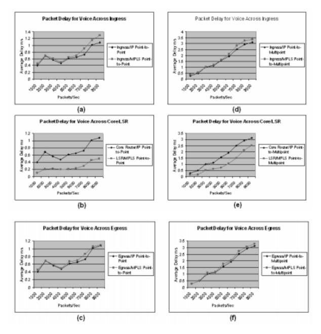
Figure 5.7 Per Packet Delay across Ingress, Core and Egress routers for voice traffic which is accompanied by background traffic.
