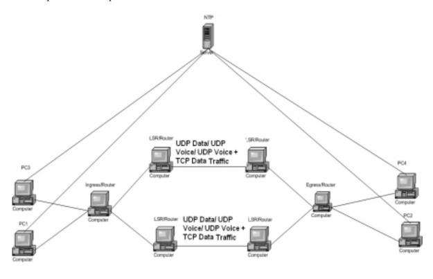
Figure 4. 1 Experimental Testbed Network.
