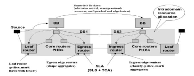
Figure 2.2 Main components of a DiffServ Network [9].
