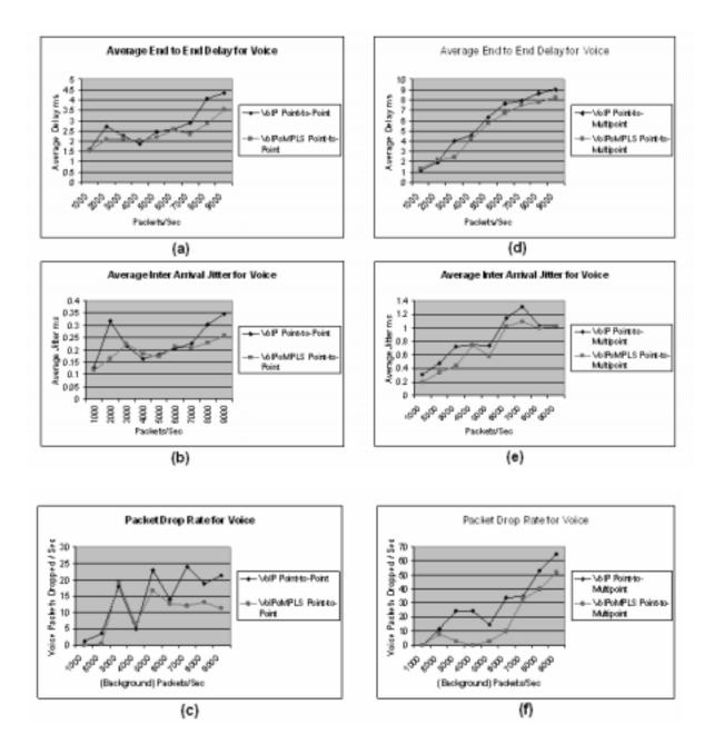
Figure 5.6 Average End-to-End Delay, Inter Arrival Jitter and Drop Rate for voice traffic that is accompanied by background traffic.
