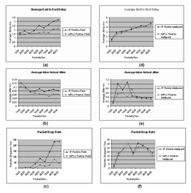
Figure 5.5 Average End-to-End Delay, Inter Arrival Jitter and Drop Rate for only UDP traffic.
