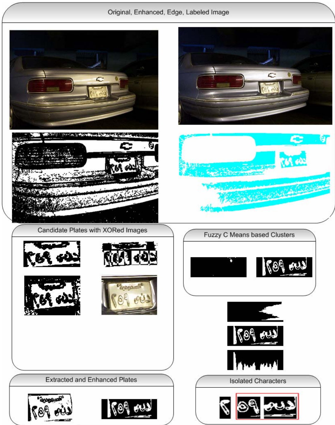
Figure 7-7: Failure case: Image taken under extreme low light with artificial illumination directly incident over a bent plate (VA implementation)
