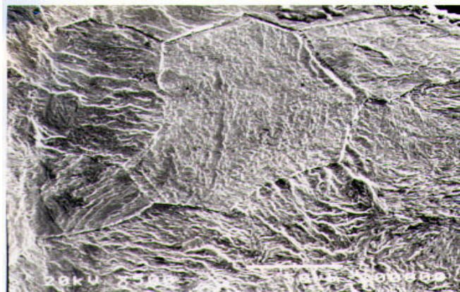
Figure 15. Another brittle fracture view of the same sample in figure 13, 500X.
