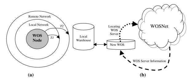
**Figure 3:** (a) **T1:** Initially, a message is broadcast to machines in the current local Network. **T2:** In the case where no local host responds to the initial request, a message is broadcast to hosts located in the next network level. (b) WOSRP Information Retrieval Strategy.
