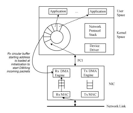
Figure 1. Architecture model of DMA-based design
