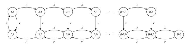
Figure 3. Markov state transition diagram for modeling interrupt disable-enable scheme
