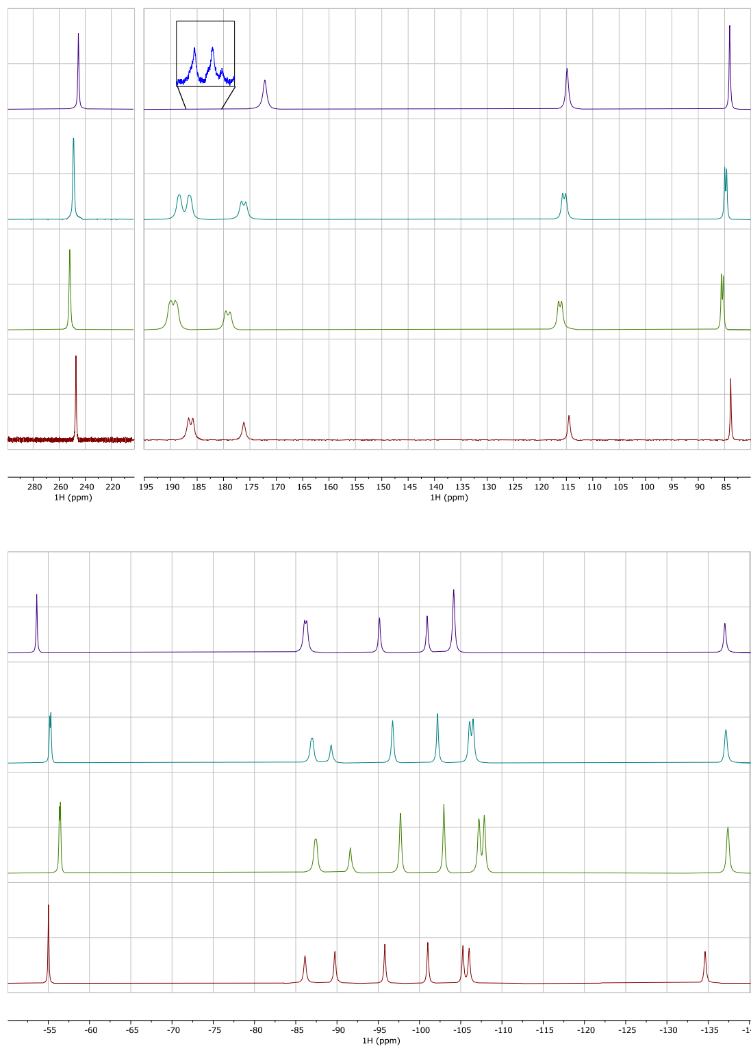
Figure S86: Stacked upper and lower range of the Yb-DOTA-M7FPy spectrum. The spectra were recorded at different pH values (blue pH = 1.2, green pH = 1.6, red pH = 6.1, black pH = 6.5) and containing different ions. Blue and green contained TFA. For red the TFA was removed by Sep-Pak column chromatography and the sample was buffered with 50 mM phosphate buffer. For black the TFA was removed by Sep-Pak column chromatography and the sample was measured in “neutral” \text{D}_2\text{O} .
