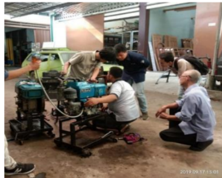
Fig. 4. Opacity test using smoke opacimeter
