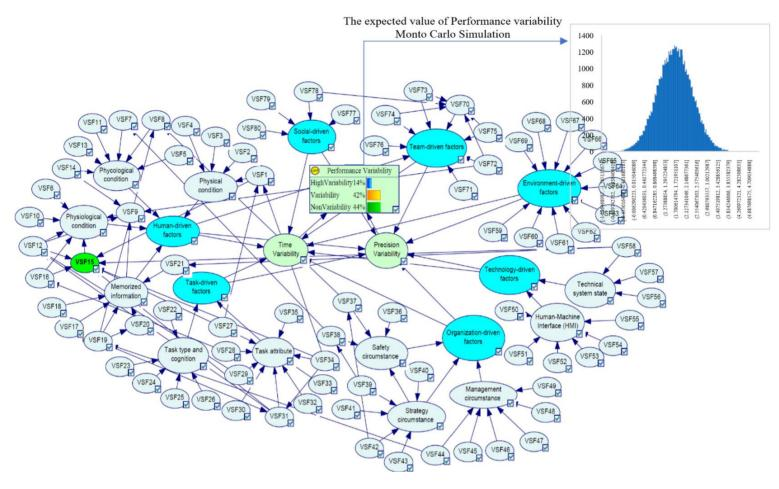
Figure 4. 6 The probabilistic causation model for performance variability of Function#18 (*Conducting the Pre-Startup Safety Review (PSSR) and run operation*)
