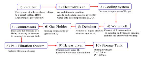
Figure 3. 2 A block diagram of hydrogen generation plant by alkaline water electrolysis.
