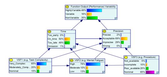
Figure 4. 3 A simple Bayesian probabilistic influence model of a hypothetical function output variability
