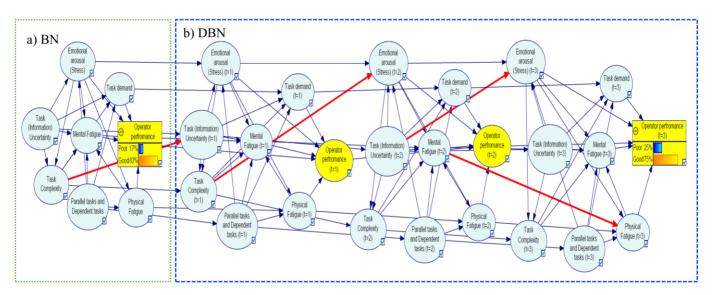
Figure 4. 9 Unrolled dynamic mutual cause-effect dependencies modeling using DBN
