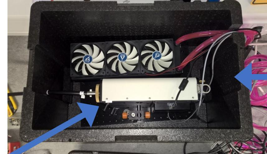
Enclosure with controlled air-temperature
