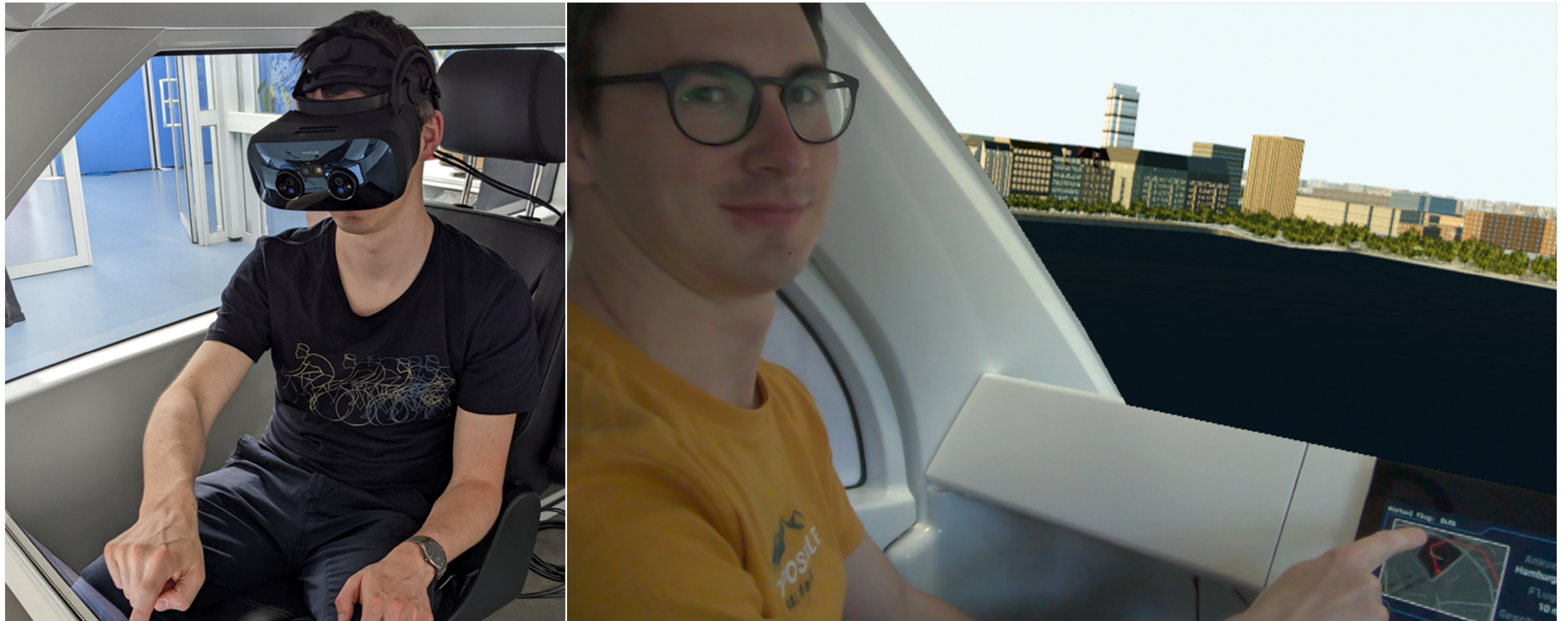
Left side: View on the participant wearing the mixed-reality hardware within the air taxi cabin. The right side shows the view the participants experienced during the flight with a steward on board. Whilst the person and the display in front of the participants are real world objects, the view outside the cabin shows the virtual flight over the city of Hamburg.
