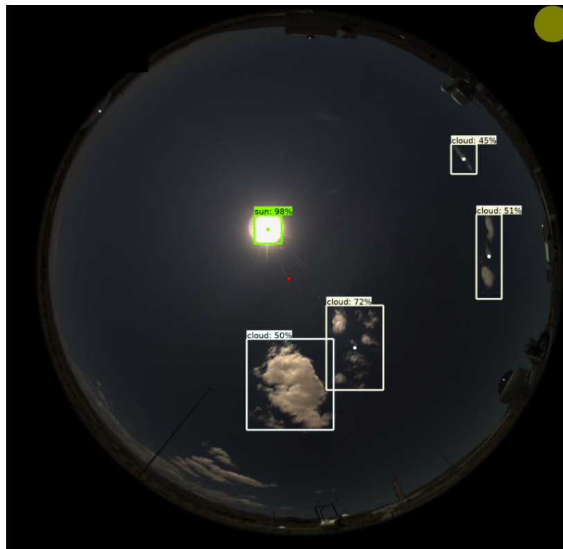
Figure 9. Object detection results from a Mobotix Q25 camera image.
