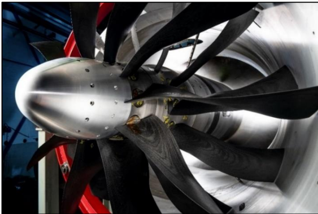
Fig. 3. CRISPMulti fan mounted on the test rig
