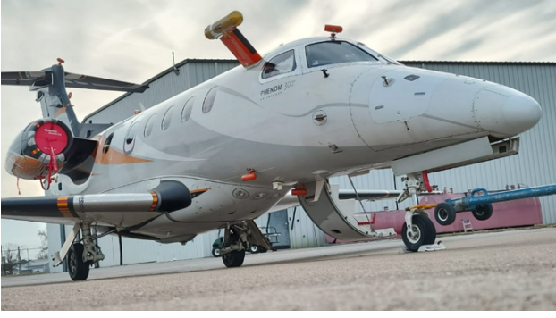
FIG 3. Embraer Phenom 300 flight test bench: prototype aircraft with all modifications for the SENS4ICE North America flight test campaign (credit Embraer).
