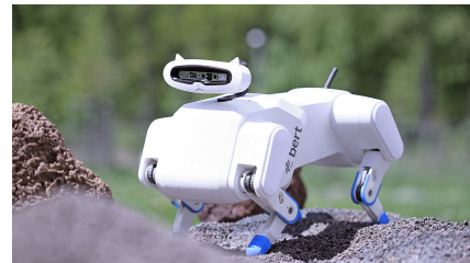
Fig. 1. The compliant quadruped Bert developed by the German Aerospace Center in a realistic field scenario.
