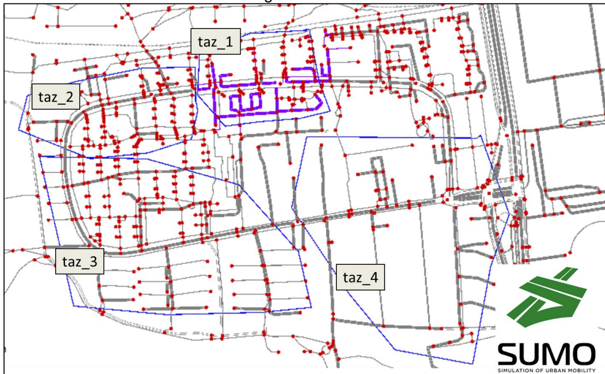
Figure 1: The examination area Schwarzer Berg with defined Traffic Assignment Zones (TAZ) in SUMO Netedit
