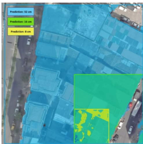
Fig. 3. Prediction effects of the field of view in dependency of the geometric resolution (yellow: 8 cm, green: 16 cm, blue: 32 cm).
