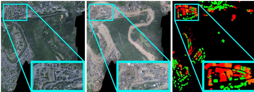
Fig. 4: Building extraction and damage assessment results on an area from the Ahr Valley, Germany. Building damage color coding: green no damage, orange damaged and red destroyed.
