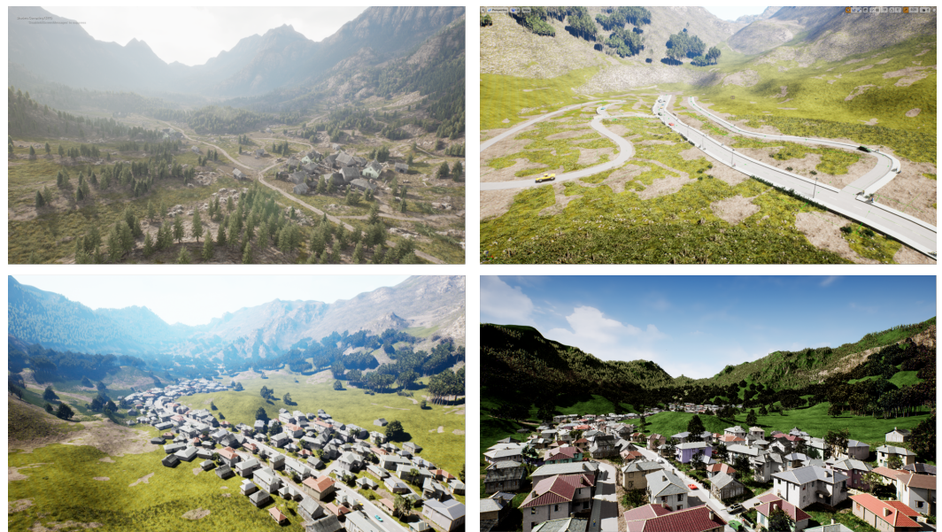
Figure 3. Steps to create the environment for the synthetic image dataset. From top left to bottom right: starting from a previously created environment ( top left ), inserting a road network and other objects ( top right ), creating various houses and inserting larger forests in the background ( bottom left ), adjusting the brightness and color tones ( bottom right ).
