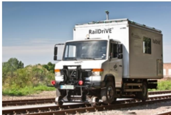
RailDrive, one of the measurement vehicles. Source: DLR-TS; CC BY 3.0
