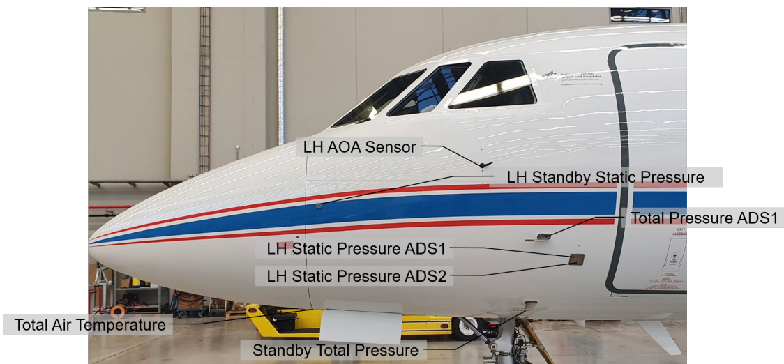
Fig. 2 Location of the ISTAR standard avionic air data sensors.
