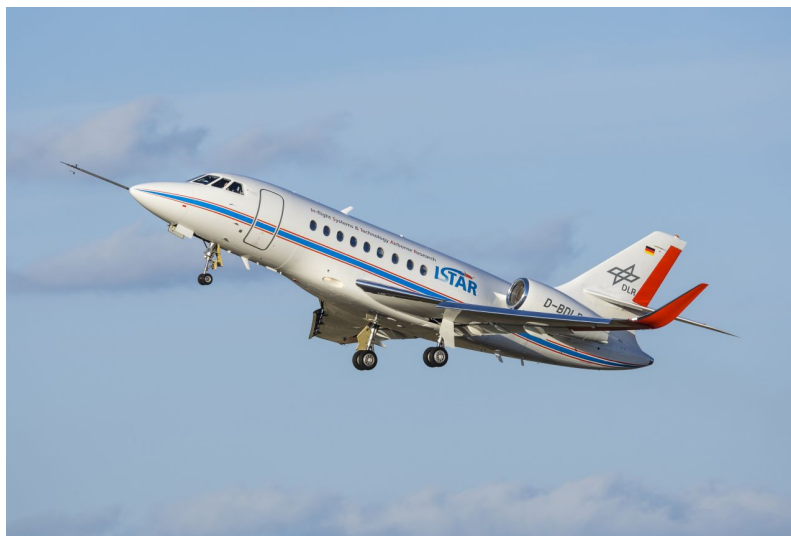
Fig. 1 The DLR research aircraft ISTAR with installed nose boom. Credit: Uwe Bethke.
