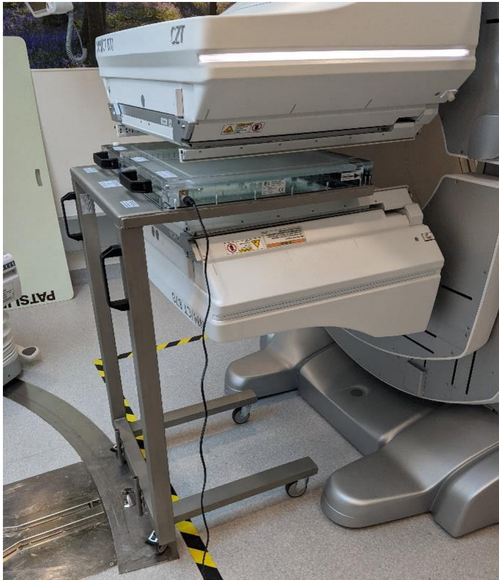
Figure 26: Gamma camera set up for the uniformity calibration and test using the fillable flood phantom with inbuilt mixer placed on the positioning cart
