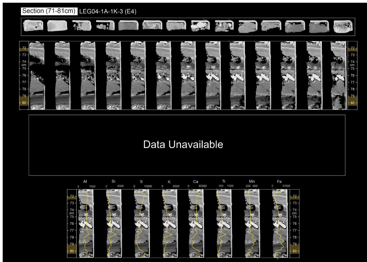
Figure A3.18 – Elemental XRF data and CT scans of microbial mats in sediment core LEG04-1A-1K-3 in Lake Estanya.
