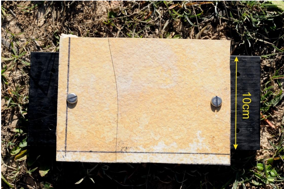
Figure 3.10 – Photograph showing a limestone slab ready to be installed in Laguna Salada de Chiprana during a field season in March 2019. Slabs were dug into the sediment at the interface with microbial mats and their position marked using a 1.5m measuring pole and GPS locations.
