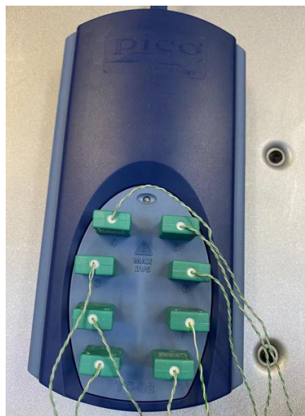
Figure 3.5 K-type thermocouples connected to Pico TC-08.
