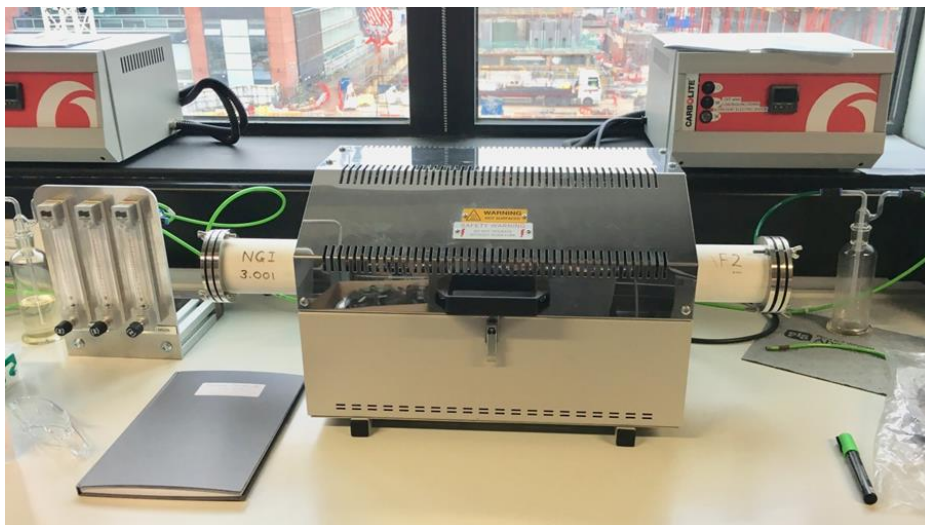
Figure 28: Furnace with ceramic tube used for reduction of rGO.
