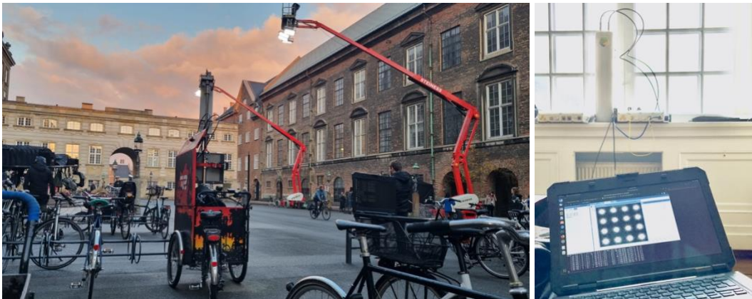
FIGURE 9: LEFT: NETWORK IN A BOX ON A BIKE – OUTDOOR CELL DEPLOYED FOR MAXIMUM MOBILITY. RIGHT: MEASURING THE RF CONSTELLATION (QAM-16).
