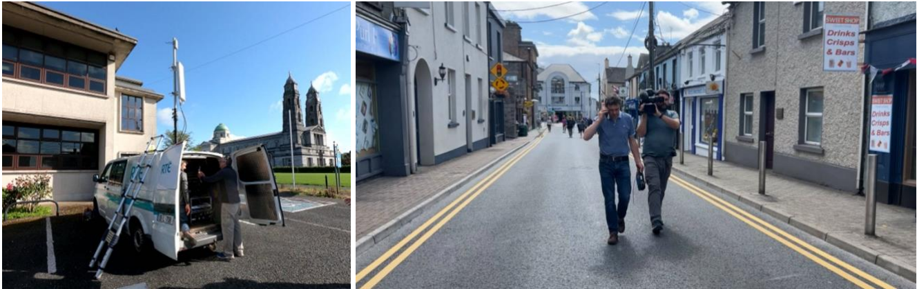
FIGURE 3: LEFT: RTÉ OB VAN WITH RADIO HEAD AND ANTENNA MOUNTED WITH STARLINK TERMINAL ON THE ROOF. RIGHT: CAMERA OPERATOR ROAMS THE STREETS TESTING THE COVERAGE PROVIDED BY THE SNPN.
