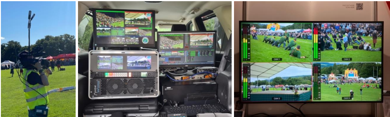
FIGURE 6: LEFT: QTV CAMERA OPERATOR WITH 5G-CONNECTED ENCODER AND ANTENNA MOUNTED ON CAMERA. CENTRE: ON SITE PRODUCTION IN THE BACK OF A LAND ROVER. RIGHT: THE MULTIVIEWER FEED RECEIVED AND DISPLAYED AT THE IBC 2022 SHOW IN AMSTERDAM.
