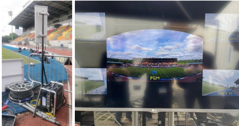
FIGURE 2: NEUTRAL WIRELESS NIB PITCH-SIDE AT STONEX (LEFT), AND THE 5G AND COFDM CAMERA FEEDS (RIGHT).
