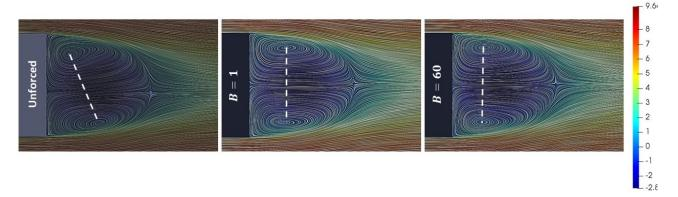
Figure 5.9: Streamlines based on the time-averaged streamwise velocity projected on a plane at mid-height of the body. The unforced case is shown on the left and the controlled case with B=1 and B=60 are shown on the middle and the right, respectively.
