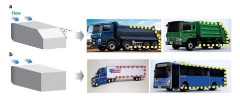
Figure 2.2: The general models of the canonical Ahmed body and the most relevant real road vehicles. The fast-back with the slant angle of  $\alpha$  is shown in (a) and the square-back with  $\alpha = 0$  is shown in (b), adapted from Choi et al. (2014).
