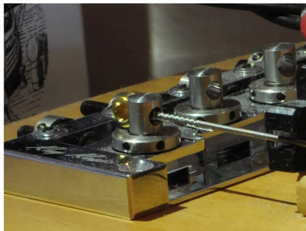
Fig 3. Ray Ross bass guitar bridge. The string is installed such that both a portion of the loop of core wire (that passes vertically over the ball end), and the knot that ties the core onto the ball end, form part of the sounding length of the string.
