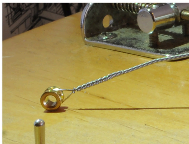
Fig 1. String. The bass guitar string, nominally 0.045 inches diameter and designed for G_2 pitch, seen uninstalled from the instrument.
