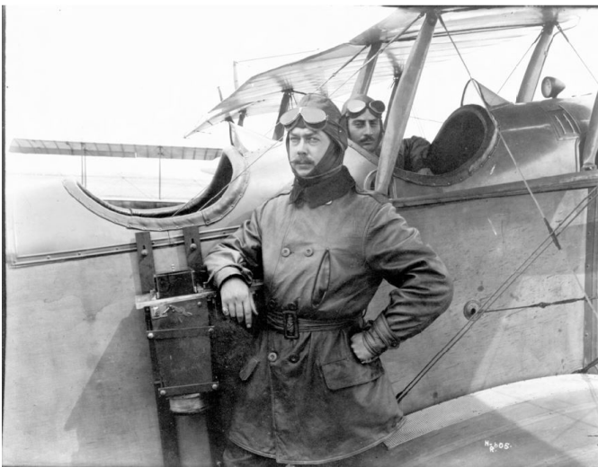
(b) American Biplane Curtiss JN-4 with external mount for aerial cameras.
