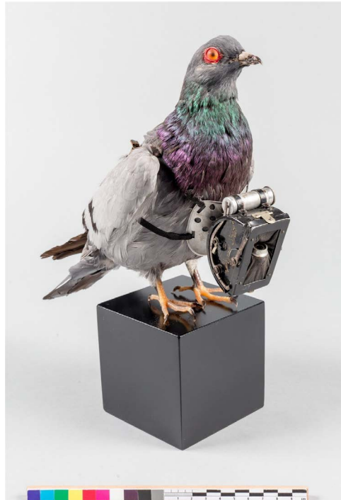
FIGURE 3.51: Julius Neubronner's 1907 Doppel-Sport Panoramic Camera (portrait format, size of the camera: 44 \times 70 \times 40 mm).
