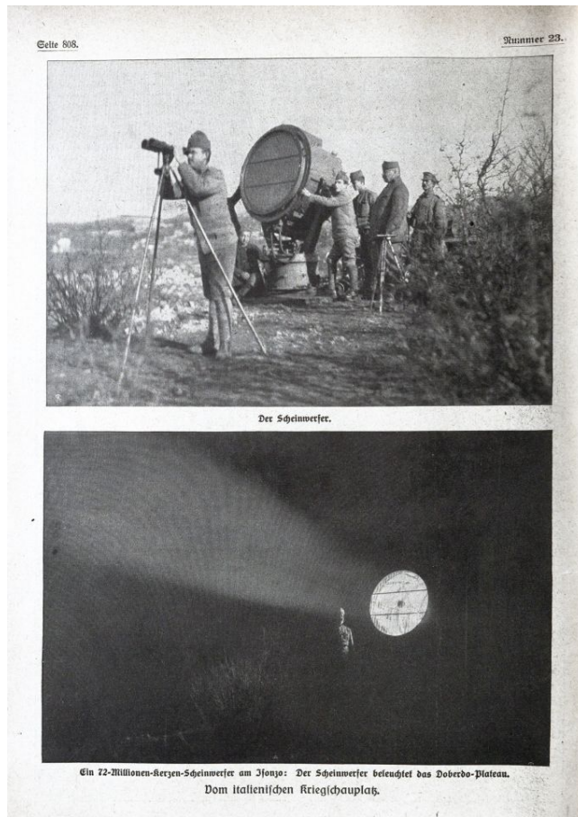
FIGURE 3.37: A 72-million-candlepower searchlight on the Isonzo (Soča) River that illuminated the Doberdo Plateau in the Italian front ( Die Woche 1916a, 808).
