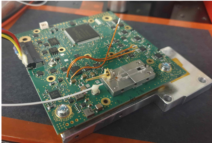
Figure 3.6: The sender flight model before the optical bench has been covered by an aluminum housing. The fully assembled flight model is shown in figure 6.1.
