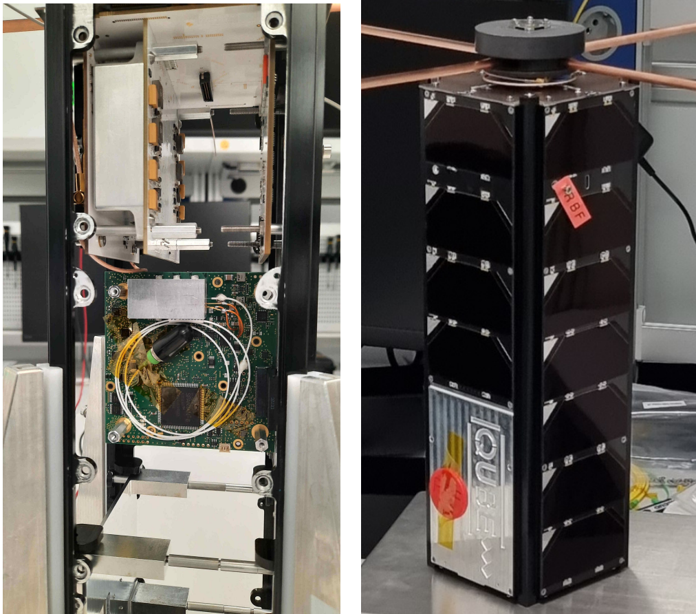
Figure 6.1: (Left) The LMU QKD sender FM (LMU FM) as the first payload and in general one of the first parts integrated in the QUBE FM. At this stadium, the LMU FM has been mechanically fixed and electrically connected via the UNISEC [67] interface. The optical fiber has been temporarily fixed on the board and the dedicated clock line, which is to be connected to the socket at the bottom right of the LMU FM, has not been attached yet. (Right) The fully integrated QUBE satellite FM. The red cover on the bottom protects the opening of the star tracker sensor.
