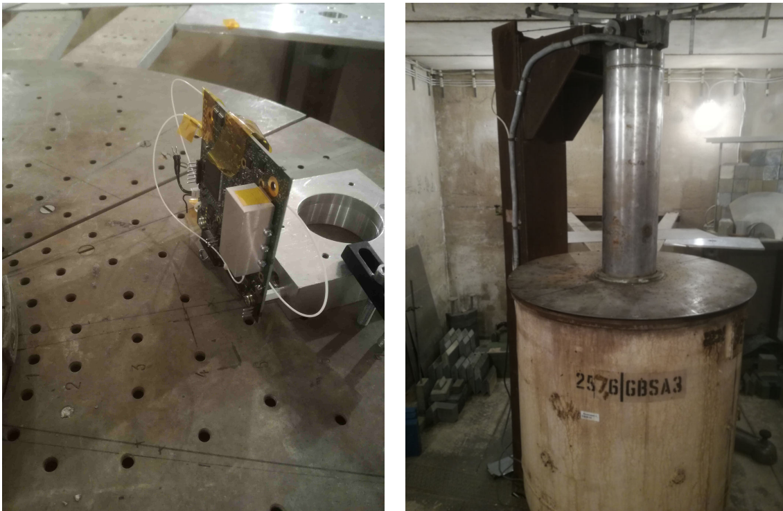
Figure 4.1: The QKD sender EQM (left) in the TID test facility at the Helmholtz Center Berlin (right). The applied dose depends on the distance to the Cobalt-60 source as well as on the duration of irradiation. During a three-day campaign various dose rates were set with hardware switched-off during irradiation and intermediate short functional tests.
