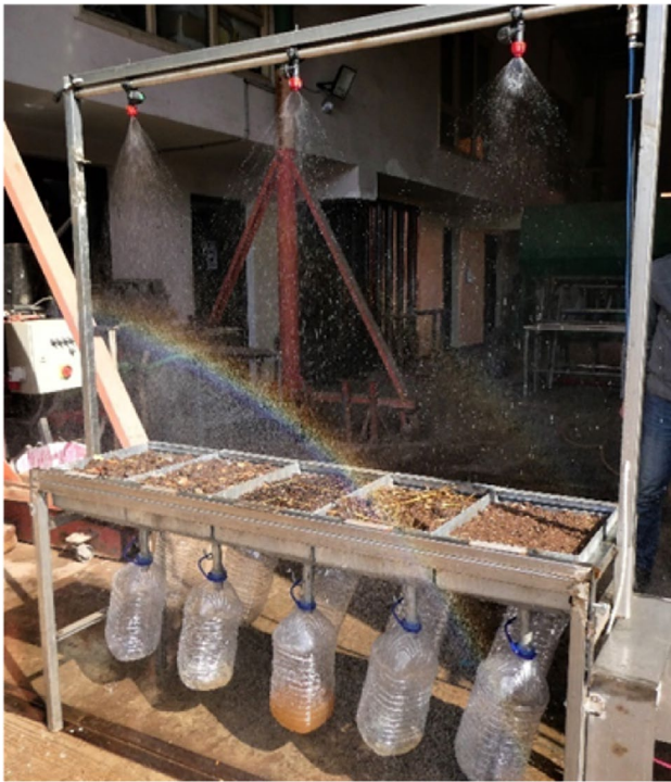
Figure 5 Rainwater simulator developed by INRA is being tested before the Farmer Field Schools (FFS) in Settat, Morocco. Source: Harun Cicek.
