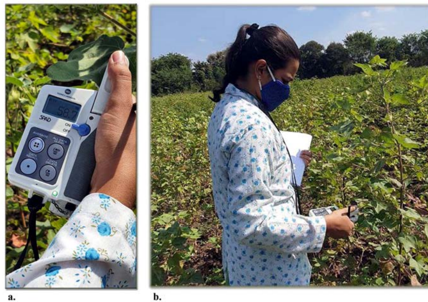
Figure 3. Use of SPAD 2.0 meter for measuring chlorophyll content. Note: (a) The digital SPAD 2.0 meter displaying the chlorophyll content of 58.7 in the cotton leaf. (b) Observations being taken on the field with the use of SPAD 2.0 meter at 60 DAS (days after sowing).
