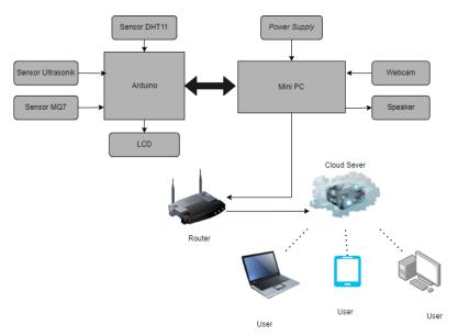
FIGURE 3. Block Diagram of Monitoring System
