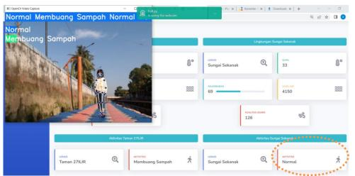
FIGURE 7. Normal Webcam Detection Results on the River
