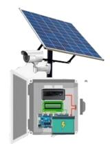
FIGURE 4. Monitoring System Hardware Design
