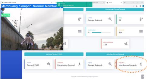
FIGURE 6. Webcam Detection Results of Littering in the River
