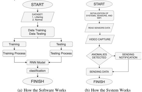
FIGURE 2. Flowchart of How the Software Works and How the System Works
