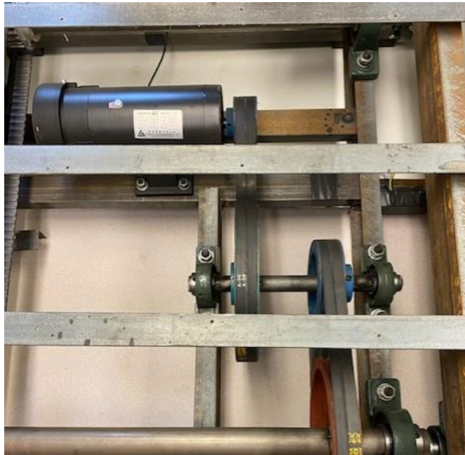
Figure 21. Location of Old Motor. Note the plane that the pulley system is on
