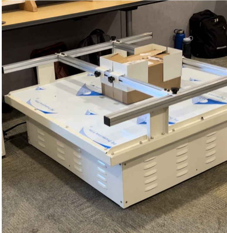
Figure 31. Example of a Package Secured During Vibration Testing
