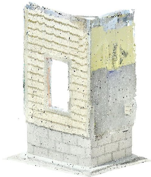
Figure 5: Screenshot of the point cloud from Figure 4 cleaned and ready for modeling in Revit.
