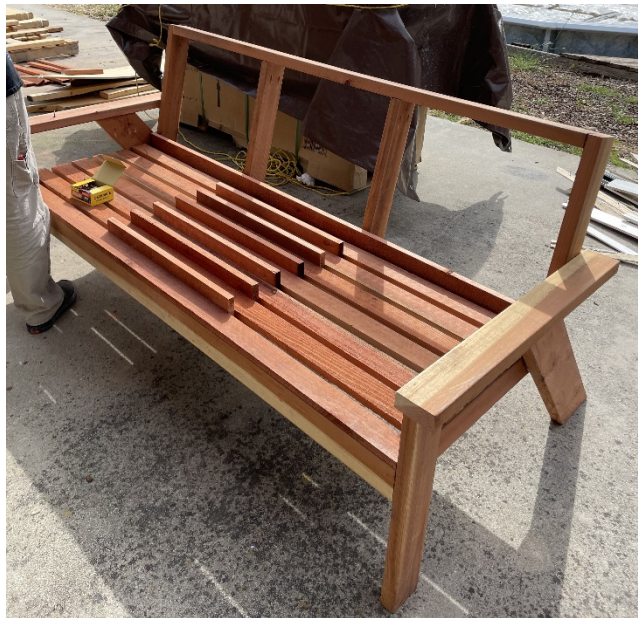
Image 7: Spacing of Seat Slats
