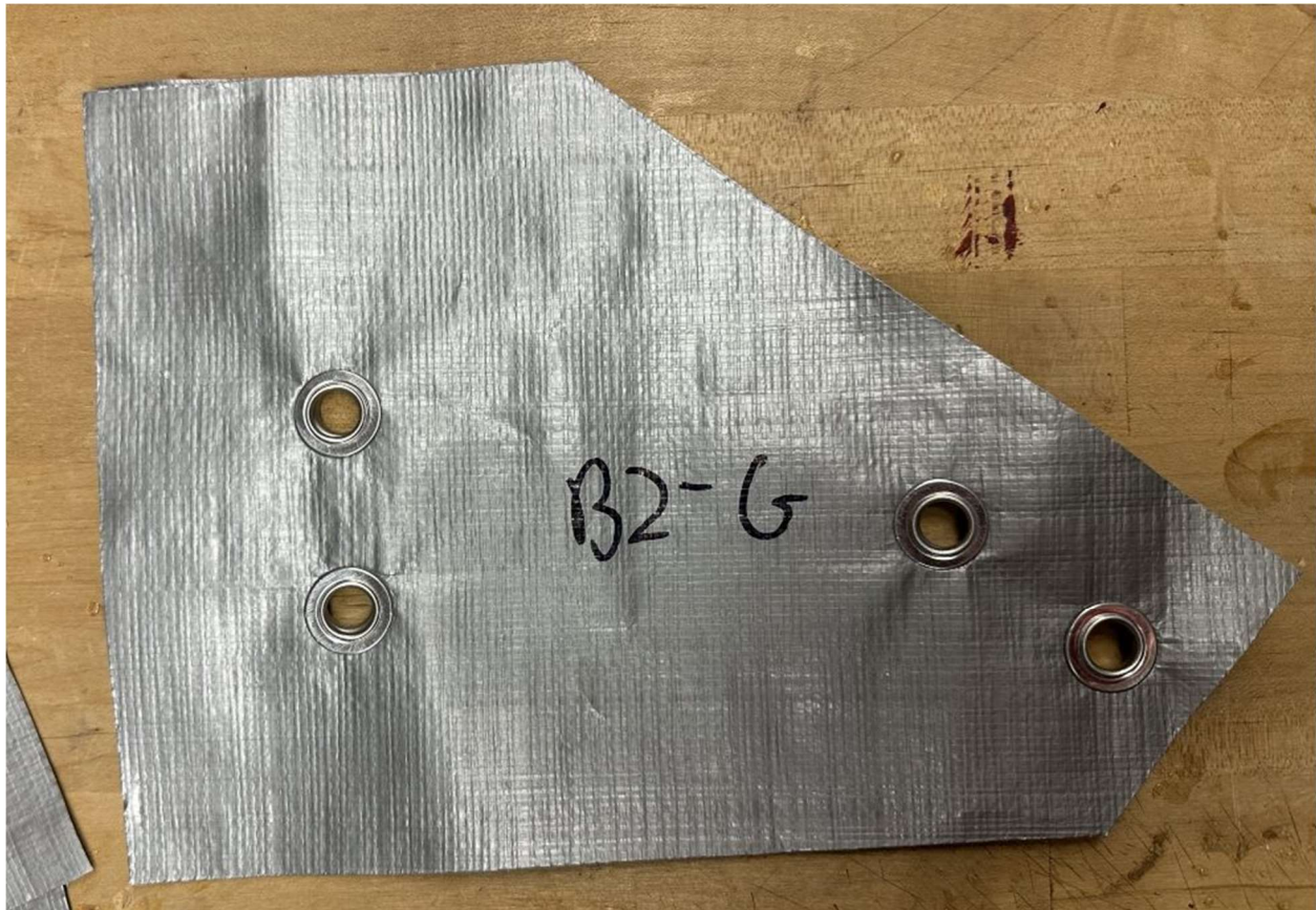
Figure 5: Physical Gusset Template
