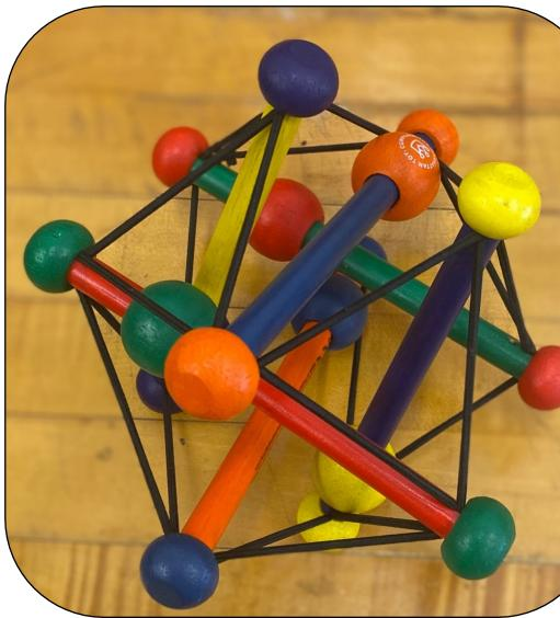
We constructed various tensegrity archetypes to gain intuition about manufacturing tensegrity and understanding tensegrity structural behavior. We discovered certain opposing directional forces that would cause tension and slack on opposing rods and impact the whole structure's integrity. Patterns of triangulation and having at most two tension lines per node appeared through this and were employed in an iterative design process.
