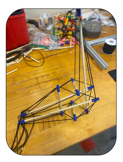
Purpose: To be paired with a spool or pulley mechanism to lengthen or shorten the cables to create tension in the tensegrity exoskeleton when the arm is moving in a specific direction.
