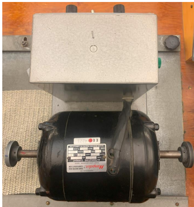
Figure 10: Hampden SM-100 Synchronous Machine
