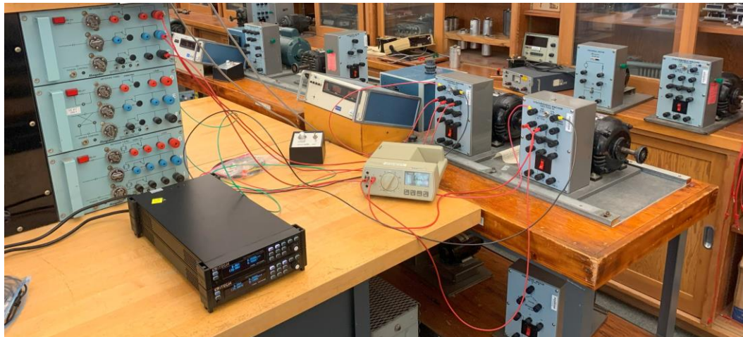
Figure 30: Open Circuit Test Experimental Setup
