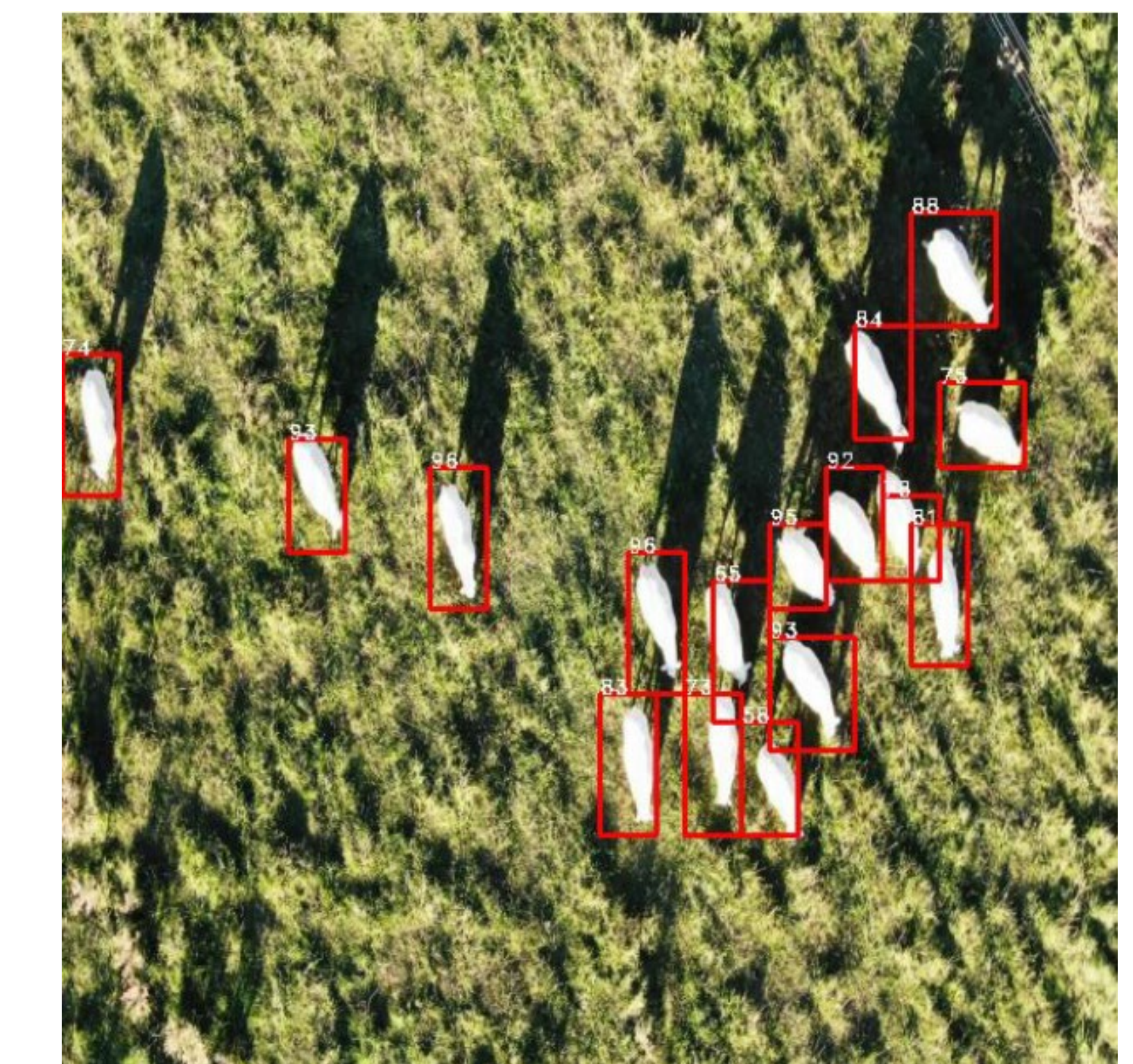
Figure 2) Faster R-CNN Object Detection Benchmark - Model is very accurate and gives exact location of sheep/cattle but is much slower and thus costs more power than hashing.
