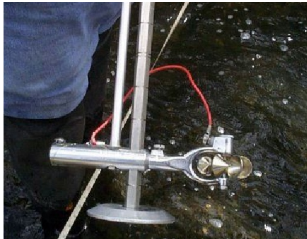
Figure 8. Pygmy meter attached to wading rod
