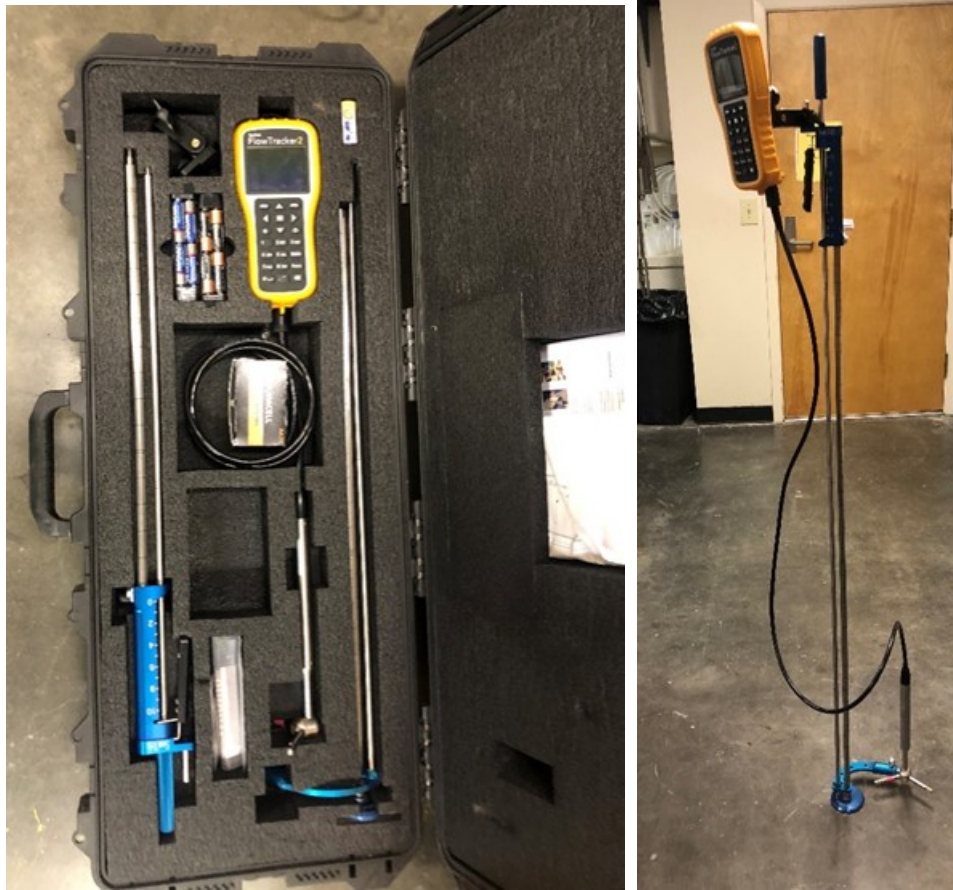
Figure 4. FlowTracker2 disassembled in portable case (left) and assembled (right)
