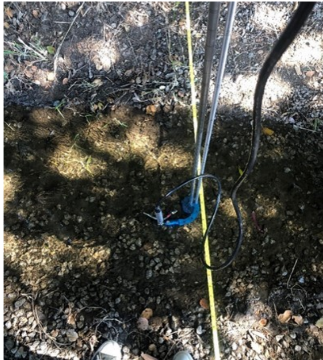
Figure 22. FlowTracker2 testing in earthen channel
