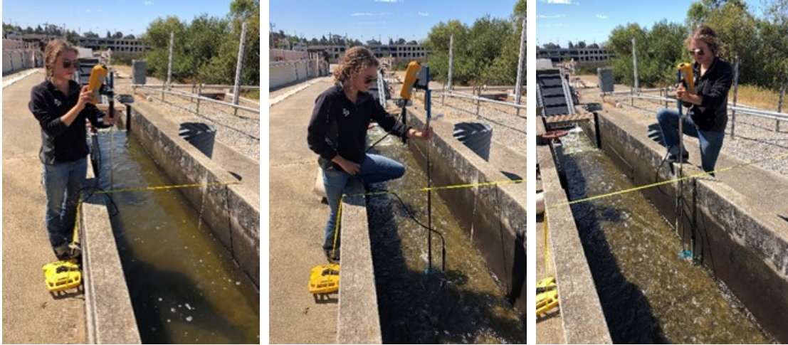
Figure 12. Left bank, center, and right bank measurements
