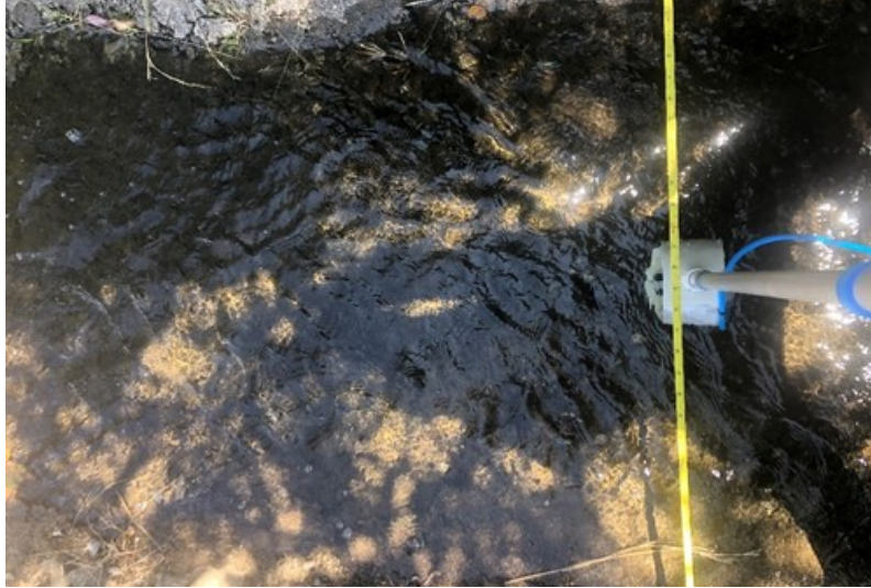
Figure 21. AgriFlo in rough concrete channel
