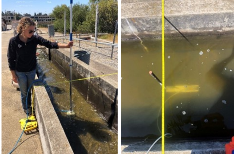
Figure 14. AgriFlo (left) and MantaRay (right) measurement
