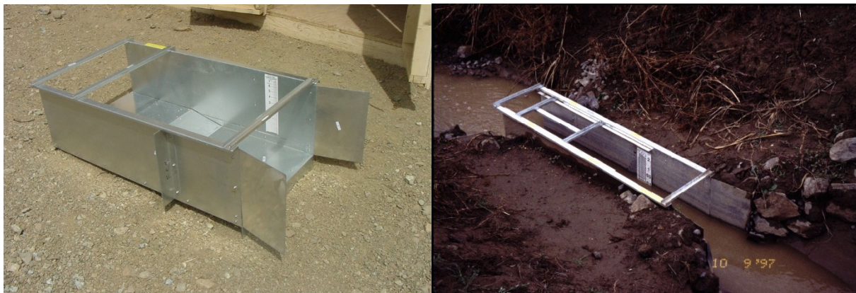
Figure 43. Portable Replogle/ramp flumes used for very accurate flow measurement
