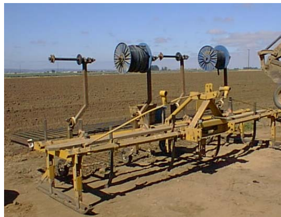
Figure 5. Tape injection unit manufactured by farmer with many commercially available parts.
