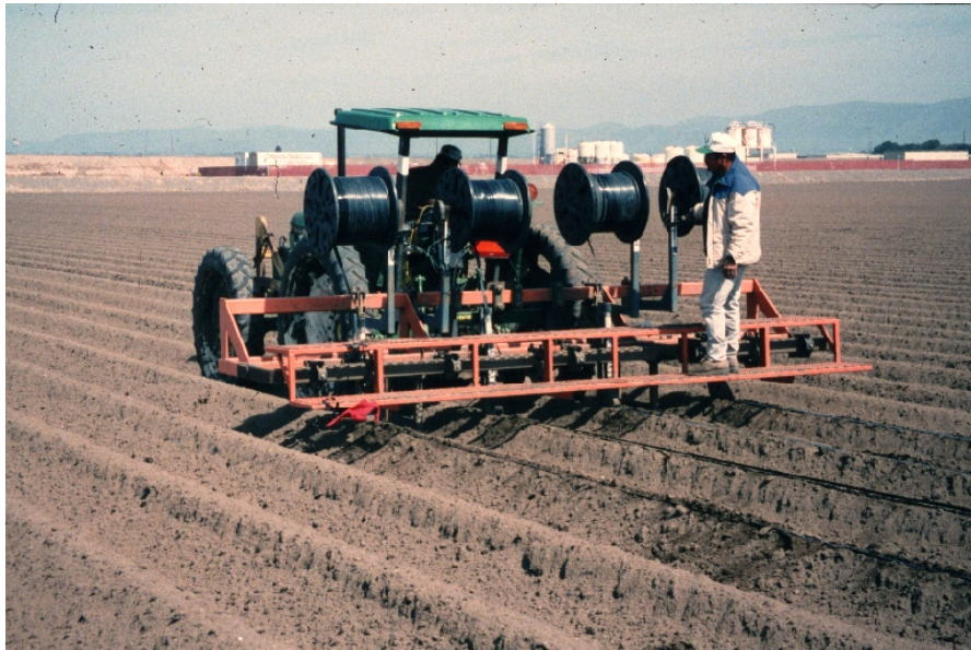
Figure 5. Tape injection unit manufactured by farmer with many commercially available parts.
