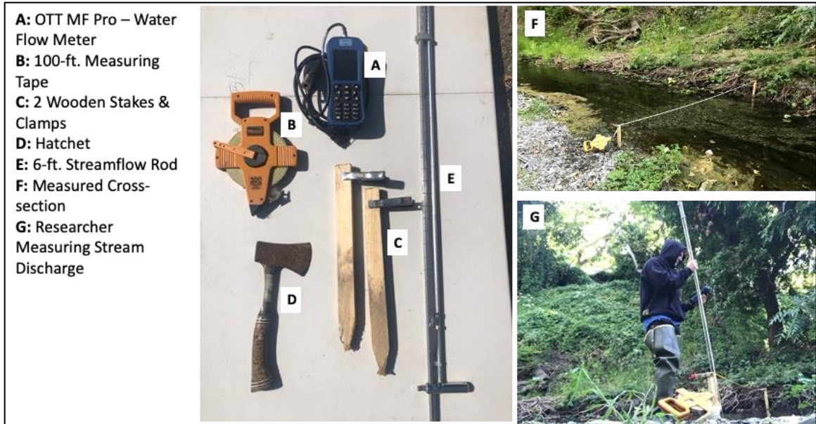
Figure 3.4 Stream discharge equipment and usage at the Lemon Orchard site.
