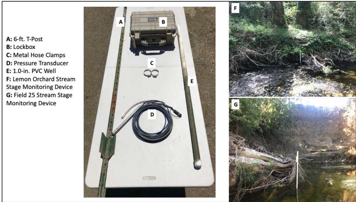
Figure 3.3 Stream stage monitoring equipment and in-stream measuring sites.
