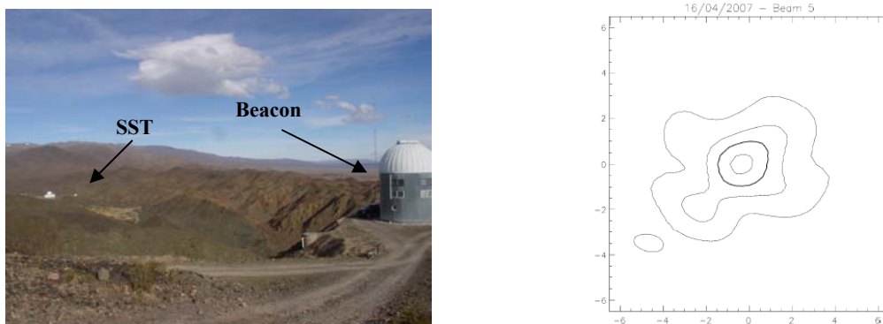
Fig. 5 The 405 GHz beacon location with respect to SST (left) and the 405 GHz antenna pattern obtained (right)
