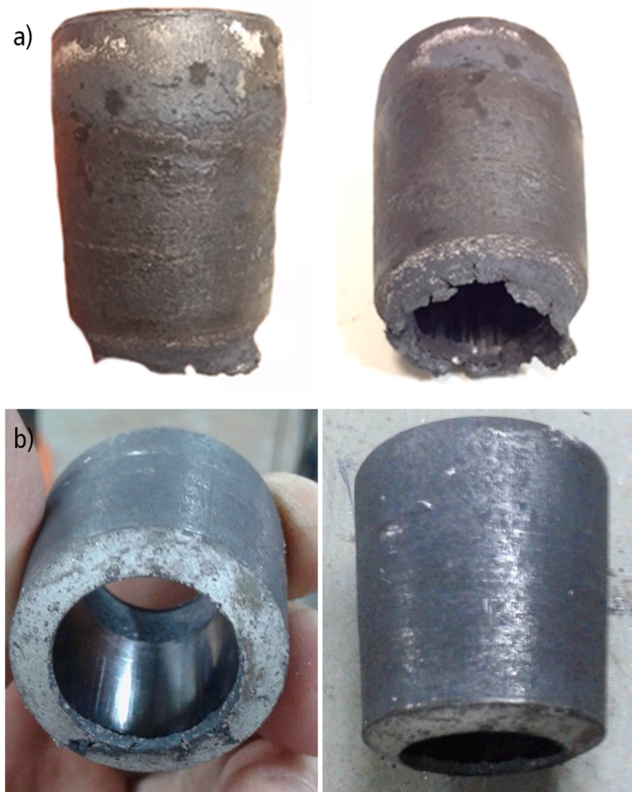
Fig. 10. Preforms obtained from: a) an unslotted billet, and b) a billet with a slot.
