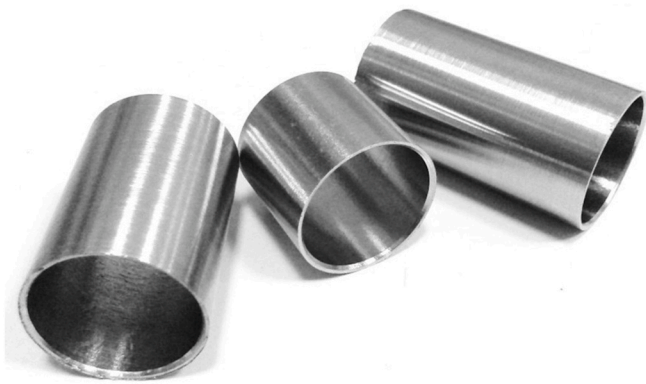
Fig. 11. Finished couplings, manufactured by PE and final machining.
